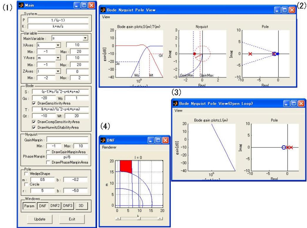
Fig. 3: A screen shot of parametric robust control toolbox
