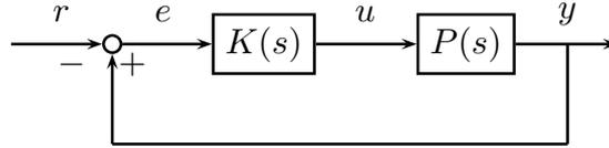
Fig. 1: A feedback control system
