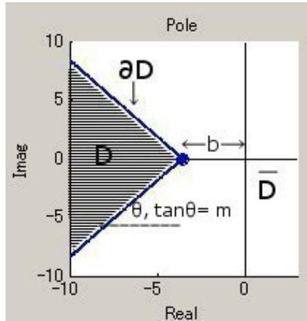
Fig. 2: Pole location(wedge shape)
